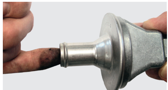
Fig. 1: Simple inspection of the non-return valve
